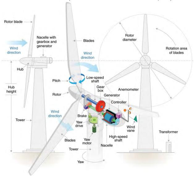
Figure 2.10.1-1. Components of a wind turbine. Source: Augustine (2012).
