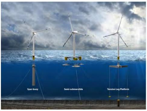
Figure 2.10.1-2. Floating offshore wind designs. Source: Department of Energy.
