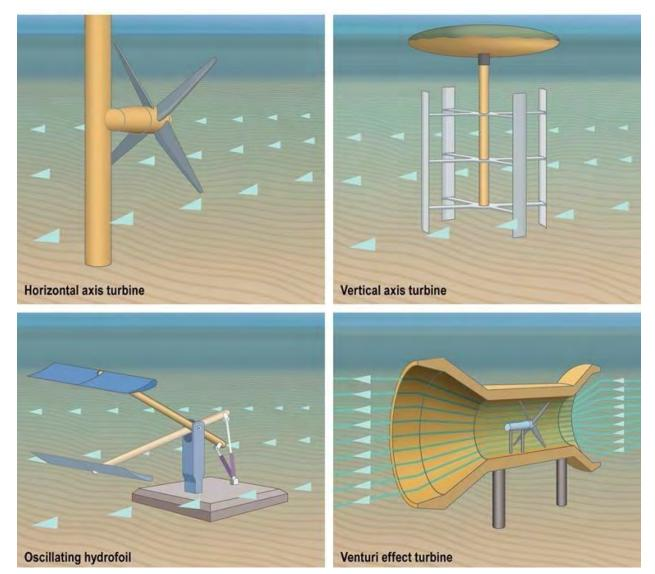
Figure 2.10.1-5. Primary technology types for tidal current energy devices. Source: Augustine (2012).
